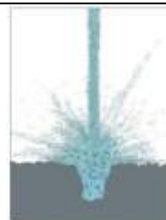
Fig. 8: Flow pattern of WJ
